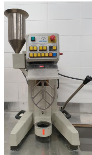
Fig. 1. Mixer M1 with the mixing bowl (a) showing the mixer head with bowl removed (b)
